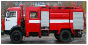
**It is intended for:** operative delivery of fire-fighting crew, equipment and fire-protection substances to the place of fire; -fires extinguishing in skyscrapers by water and foam-agent water solutions supply through high pressure hose lines
