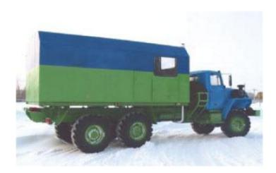
The commercial steamer YΠΠ on the chassis of the go-anywhere vehicle is intended for de-waxing well bottom zone, piping, tanks, armature and other oil field equipment with high pressure saturated steam, as well as for heating and washing the equipment.
