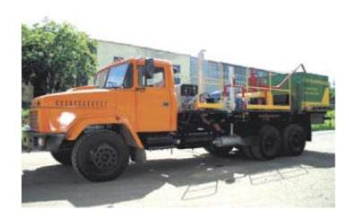
It is intended for forcing technological liquids while cementing, washing out sand plugs, hydro break of layers, drilling, capital repair as well as while doing other washing and squeezing jobs in oil and gas wells. The hydraulic part of the three plunger horizontal pump can be manufactured in different ways depending on the diameter of the installed plungers (d=100, d=110, d=125, d=140).
