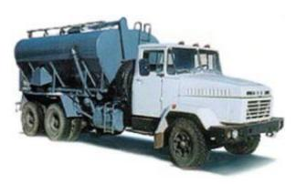
It is intended for transporting dry powder-like materials, mechanically regulated feeding of these materials by screw conveyors and for preparing grouting mortars while cementing oil and gas wells.
