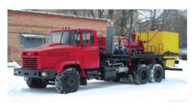
A special truck, mobile pumping truck 160x32 is intended for pumping different liquid media while cementing wells in the process of drilling and capital repair as well as while doing other washing and squeezing jobs in oil and gas wells.
