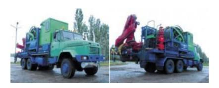
It is intended for performing technological and repair-and-renewal operations at oil, gas and gaseous condensate wells without killing them using a steel long-length flush-joint pipe. It can perform such operations as abandonment of wax sediment, hydrate and sand blocks; processing the bottom hole formation zone; doing geophysical research; installing cement bridging; doing job in insulating layers and others.
