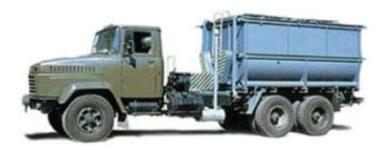
It is intended for processing grouting mortar in the process of its preparation for the purpose of reaching the homogeneity of the mixture parameters throughout its volume. The unit is used in all kinds of cementing jobs which are done in drill holes. The unit design allows to use it for preparing buffer compositions and tempering liquids.
