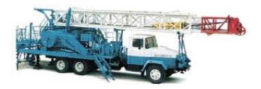
The unit AK-60n is intended for the development and repair (including capital repair) of the oil and gas wells up to 3000 m deep, located as a well cluster or separately. It allows doing drilling jobs 1600 m deep. The load-carrying capacity of 80 tons allows liquidating emergency situations at repairing wells doing without units of higher capacity. The unit is designed for work in areas with cold and moderate climate (working temperature is up to -45°C, storage temperature is up to -55°C).
