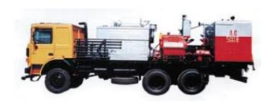
It is intended for forcing technological liquids while cementing, washing out sand plugs, hydro break of layers, drilling, capital repair as well as while doing other washing and squeezing jobs in oil and gas wells. The hydraulic part of the triplex plunger horizontal pump can be manufactured in different ways depending on the diameter of the installed plungers (d=115, d=125).
