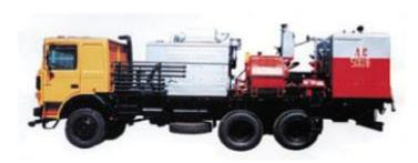
It is intended for forcing technological liquids while cementing, washing out sand plugs, hydro break of layers, drilling, capital repair as well as while doing other washing and squeezing jobs in oil and gas wells. The hydraulic part of the triplex plunger horizontal pump can be manufactured in different ways depending on the diameter of the installed plungers (0100, 0115, 0125).
