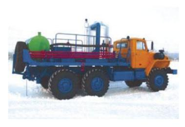
The well dewaxing aggregate A $\mu$ IIM - 12/150 on the chassis KrAZ is intended for well dewaxing with hot oil at the ambient temperature of -40°C to +40°C.
